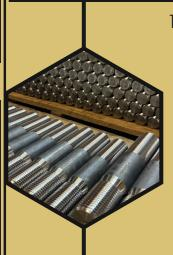
Thread cutting has been done for decades and is an efficient and very popular way to thread bolts of various sizes and lengths. Cyclone Bolt utilizes a wide variety of Landis Thread Cutting machines to keep up with the constant demand of customers requesting Double End, Tap End, and Single End studs per their print or specifications. The diameter of bar we can thread ranges from 1/4" to 2 1/2"
